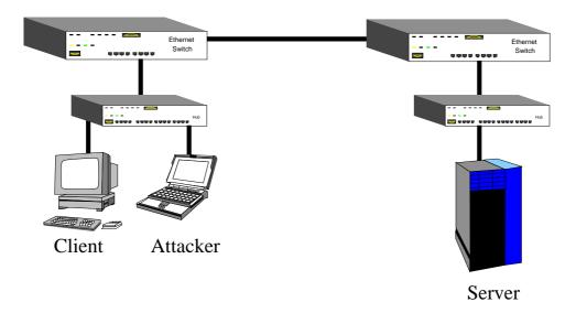
Figure 1: Server and client connected to different bridges
